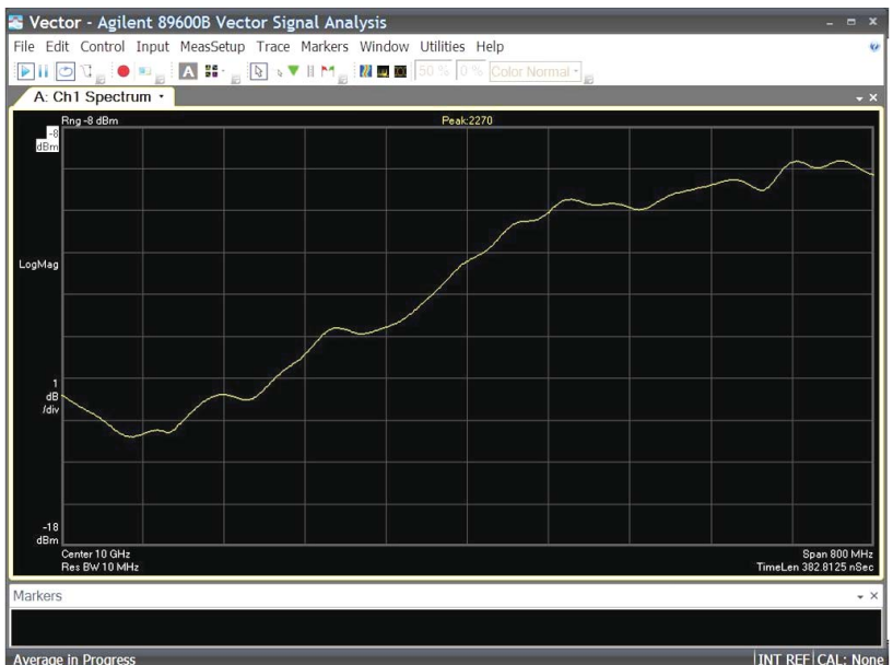
Figure 4. VSA and down converter frequency response (uncorrected)
