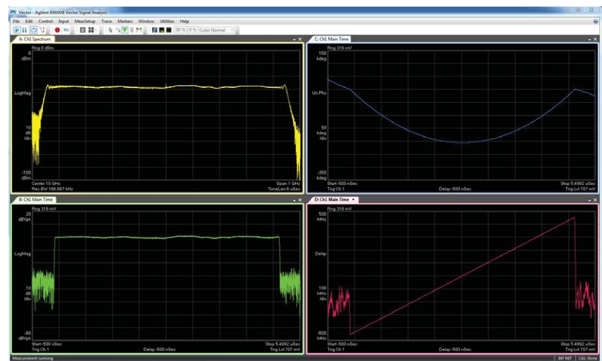
Figure 6. Example of 750 MHz chirp radar signal demodulation
